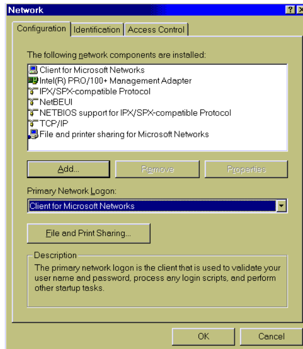
Figure 3.8 Network Control Panel in Windows 9x
