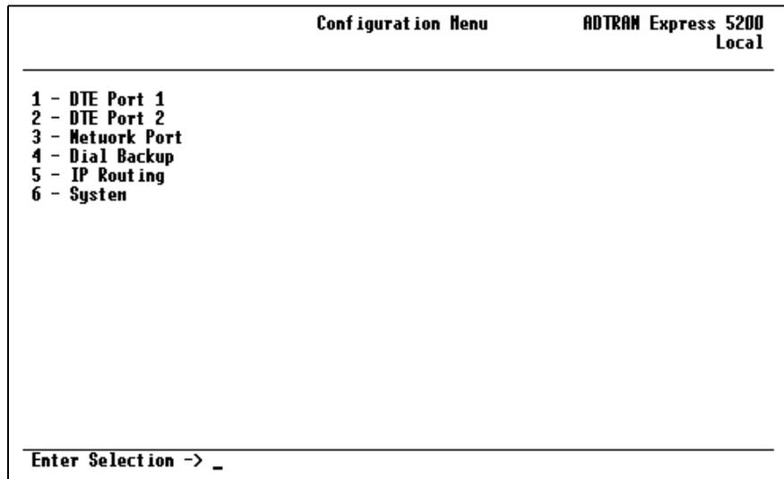
**Figure 5-1. VT 100 Configuration Menu (DBU card installed)**
