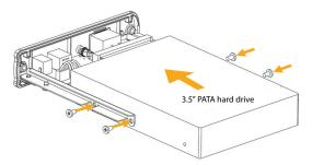
4 Slide the drive tray and drive into the enclosure.
