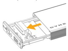
3 Connect the drive to the 40-pin data connector and to the power connector on the enclosure circuit board, then secure the drive to the rails with the four screws (provided).
