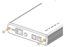
2 Remove the plastic end cap and circuit board.
