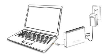
3 Press the power button to turn on the enclosure. The operating system automatically detects and sets up the new drive. The power LED turns on when the enclosure/hard drive turns on. The operating system automatically detects and sets up the new drive.
