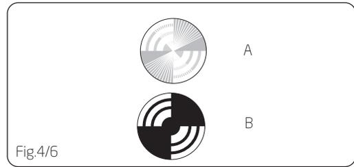
**NOTE:** If the indicator does not spin and the pattern is visible (B) when the carpet cleaner is turned ON, the brushes are not rotating.
