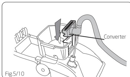
**NOTE:** Before connecting tube to cleaner, make sure black tabs are extended by pulling tan collar toward tube.
