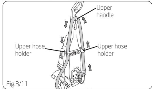
Wrap hose around lower tool holder and continue until nozzle connector is near upper hose holder.
