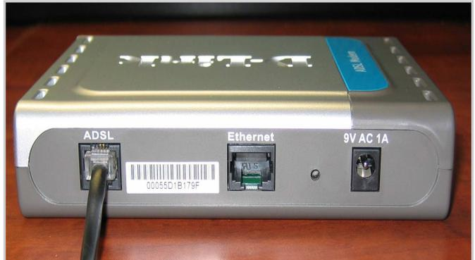
4. Connect the power adapter to the "9V AC 1A" port on the DLink modem or the "Power" port on the Comtrend modem and plug the other end into a power outlet in your house.
