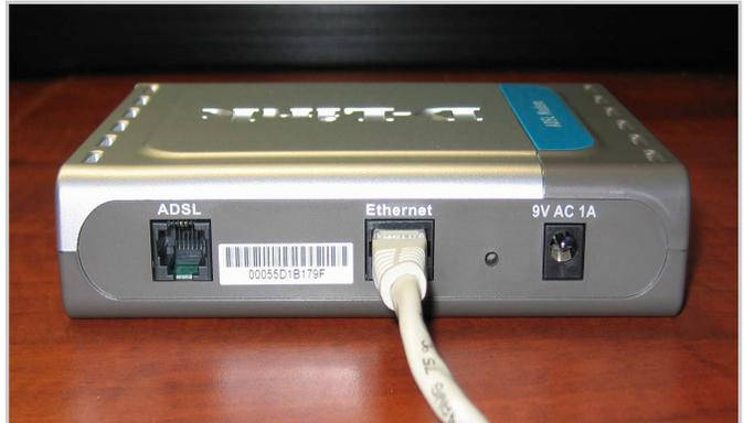
3. Now that the network cable is connected, take the phone cord that came with the kit and plug one end into the wall jack and the other end into the "ADSL" port on the DLink modem or the "Line" port on the Comtrend modem.
