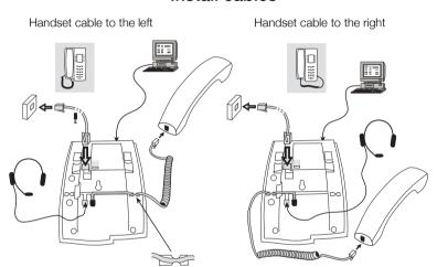
You can put the cable to the handset in the notch underneath the telephone. The cable to the exchange has to be plugged in "LINE" and the handset cable has to be plugged in "HANDSET".
