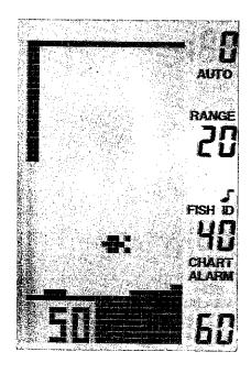
When the "Chart Alarm" signal is on, the alarm is active. If you wish to view the Chart Alarm bar, simply press the CHART ALARM key. The bar will be displayed for eight seconds. Any target that appears on the left side of the screen in the area covered by the chart alarm bar will trigger the alarm.
