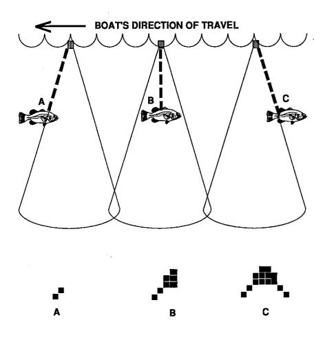
Very small fish probably will not arch at all. Medium sized fish will show a partial arch, or a shape similar to an arch if they're in deep water. Large fish will arch, but turn the sensitivity up in deeper water to see the arch. Because of water conditions, such as heavy surface clutter, thermoclines, etc., the sensitivity sometimes cannot be increased enough to get fish arches.
