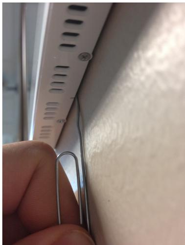
Figure 13. Paper Clip Needs to Engage Release Plate
