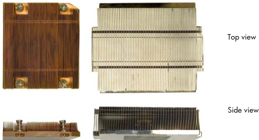
Figure 5: The left processor heat sink uses fully ducted design. The right heat sink is a traditional heat sink used in a 1U rack-mount server.
