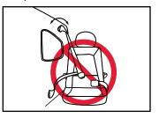
1 Vehicle belts with top or bottom anchor points on the vehicle door.
