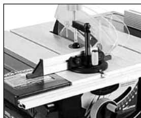
Fig 26 View of machine set for Crosscutting.
