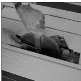
Fig 34 Close up of removing the blade using the tools provided.
