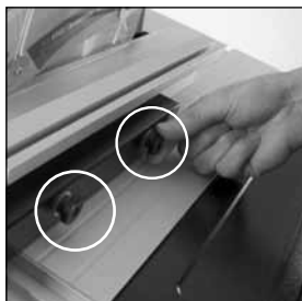
Fig 21 Close up view of the rip fence guide.
