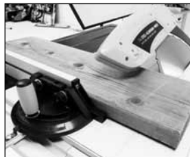
Fig 27 View of machine set for bevel crosscutting.
