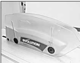
Fig 17A Saw blade in upright position with side covers deployed and touching table.
