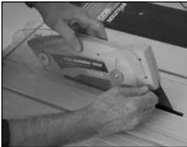
Fig 16 Close up view of the top guard being fitted.
