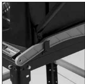
Fig 35 Close up view of push stick in its storage position.
