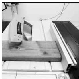
Fig 32 View of machine set for bevel rip cutting.
