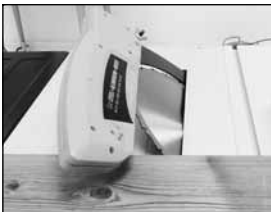
Fig 17B Saw blade tilted to discernable angle. Side covers removed.
