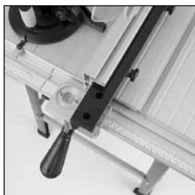
Fig 12 Close up detailed view of the fence rail being adjusted.
