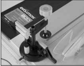
Fig 15 Close up view but with anti-bounce device fitted.
