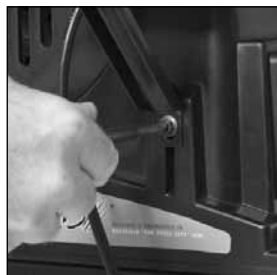
Fig 8 Close up detail. Fixing strut to turret.
