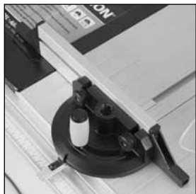
Fig 14 Close up view of mitre gauge. Anti-bounce device not fitted.
