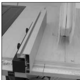
Fig 22 Close up view of the rip fence set up for LH operation.
