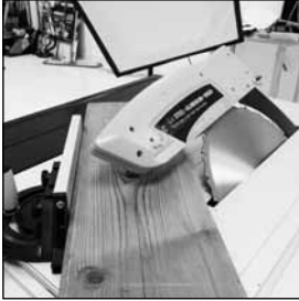
Fig 28 View of machine set for compound mitre cutting.
