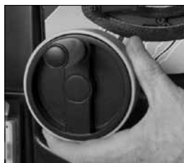
Fig 20 (B) Close up view of the tilt adjusting wheel.
