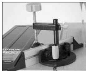
Fig 24 Close up of mitre gauge. Anti-bounce device fitted.
