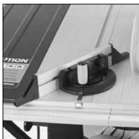
Fig 23 Close up view of the mitre gauge set to an angle.
