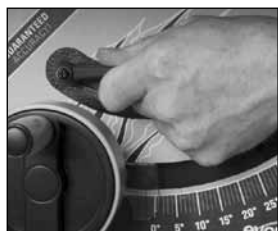
Fig 20 (A) Close up view of tilt locking lever.
