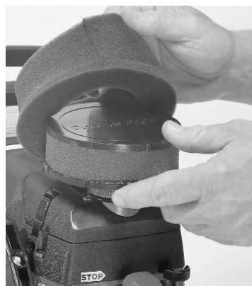
Fig. 33. Remove the Pre-filter
