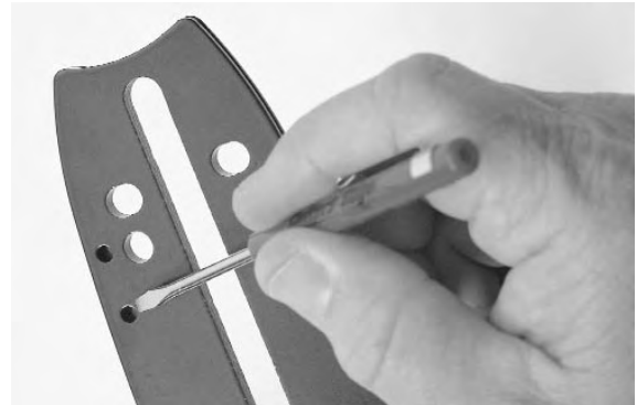
Fig. 28. Cleaning oil holes on guide bar
