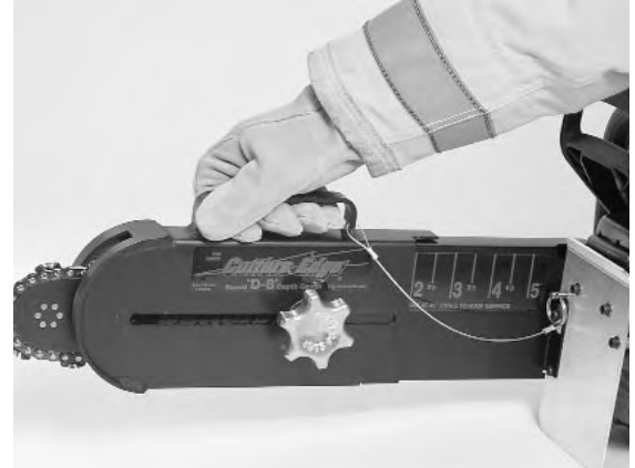
Fig. 21. Set to the desired depth of cut.
