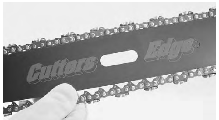
Fig. 10. Proper chain tension - while pulling chain down, drive links just clearing the rail
