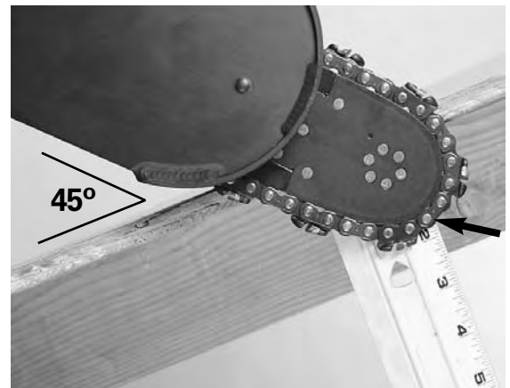
Fig. 22. Depth of cut at 45°
