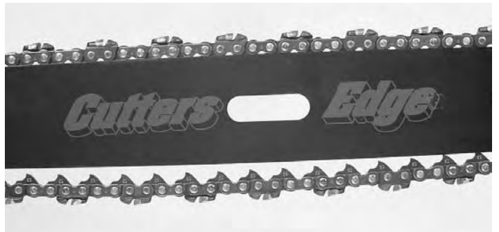
Fig. 9 "Sag" chain is too loose
