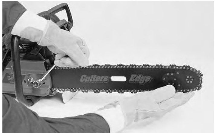
Fig. 8. Tighten two clutch cover nuts so chain is at proper tension
