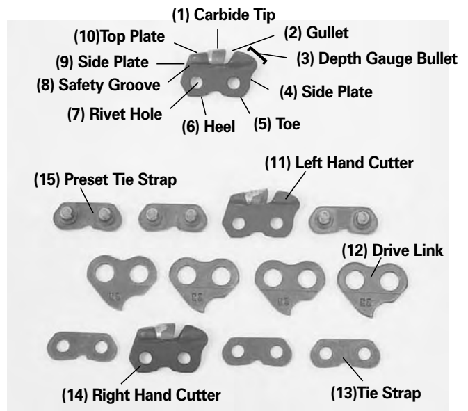
Fig. 26. Components of the BULLET® CHAIN
