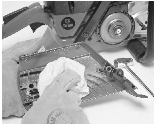
Fig. 24. Thoroughly clean the clutch cover
