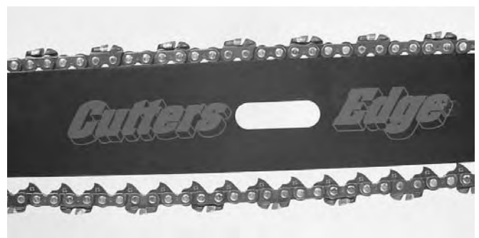
Fig. 16 The chain will sag when hot
