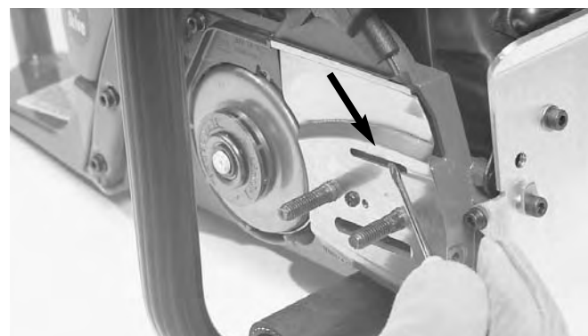
Fig. 32. Carefully clean out the oil slot
