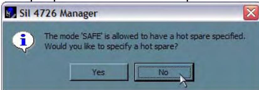
In some configurations, the end-user may want the added redundancy of a Hot Spare. The goal of this example is to use all available system capacity to deliberately avoid the Hot Spare.
