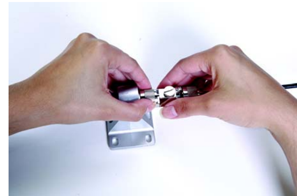
Connect the Cable to the Lightning Protector
