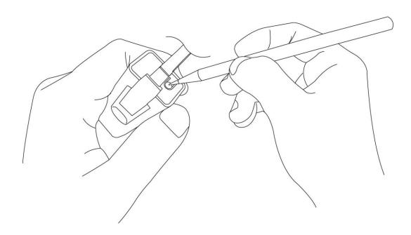
3. The LED will first stay steadily lit for approximately 10 to 15 seconds. The LED will then begin to flash rapidly for an additional 10 to 15 seconds, as the device reinitializes. When the blue LED remains lit without flashing, the device has completed its reset process, and is ready for further configuration.
