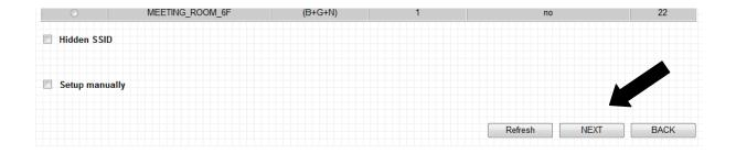
4. The travel router will save the changed settings and may reboot. If it does, reconnect to the travel router by searching available wireless networks for the device name you set in step 5 of the **Quick Installation** section. Enter the 8 to 32 character security key you set.
