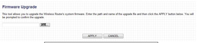
**Note**: Do not turn off or disconnect the access point during a firmware upgrade, as this could damage the device.
