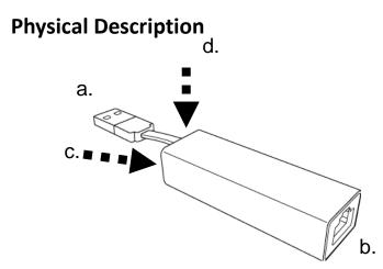
**a. USB connector and cable:** This connector can be plugged into a computer's USB port, or into a USB power adapter.
