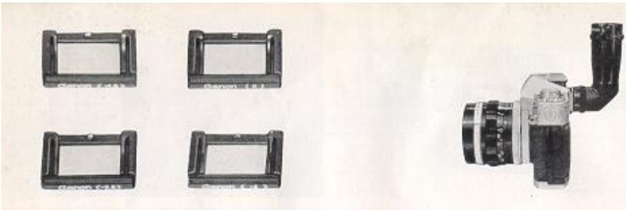
è Eyesight adjustment lenses are available as optional attachment. When an eyesight adjustment lens is attached to the eyepiece, those who are far-sighted or near-sighted can take pictures without glasses. Four different Copters of +1.5, 0, -2.5, and -4 are available.
