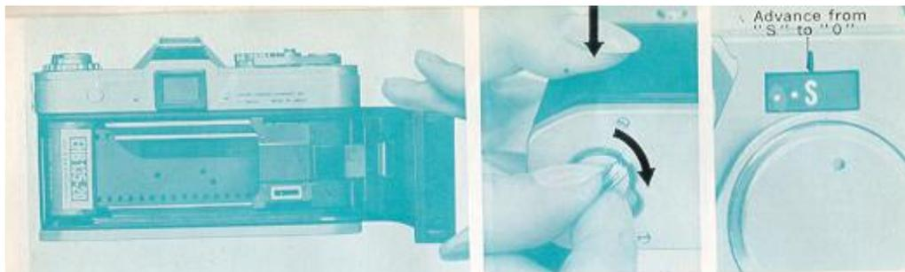
4. **When the back cover is half closed**, the QL cover presses down on the film. Check through the sprocket window whether the film has been engaged correctly onto the gear.
