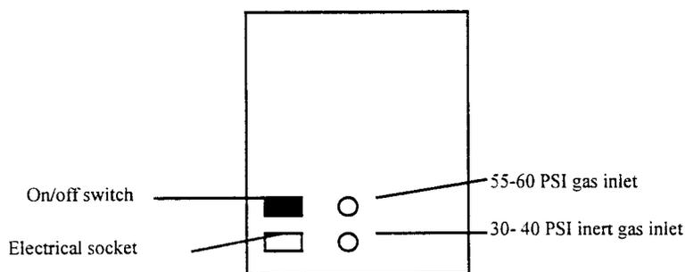
**Figure 2 - ASW Controller Unit Rear View**
