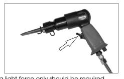
4. Release the trigger to stop operation, whilst maintaining contact with the work, noting that the tool may impact briefly after the trigger is released.
