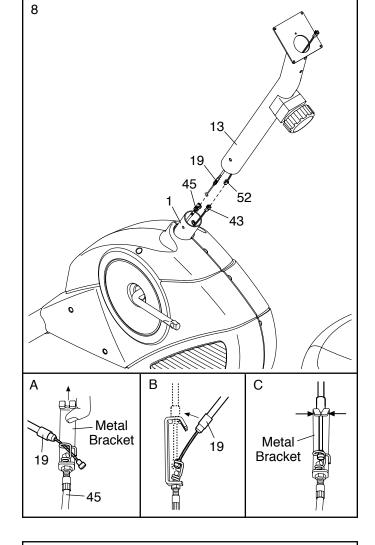
9. Insert the excess wire and cable downward into the Frame (1).
