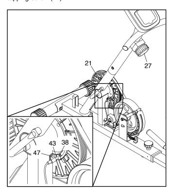
Slide the Reed Switch (43) slightly closer to or away from the Magnet (38), and then retighten the M4 x 15mm Self-tapping Screw (47). Turn the Pulley (21) for a moment.
