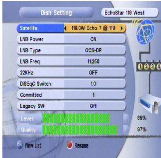
Note the green signal indicator for signal strength and quality at the bottom of the Dish Setting window and confirmation of the satellite signal being received in the upper right hand corner of the window which matches the satellite shown in the satellite browser.
