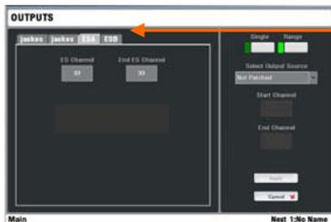
Use the Surface or Editor **OUTPUTS** page to assign sources and destinations for the EtherSound channels. EtherSound modules **M-ES-V1** and **M-ES-V2** are fully compatible and are assigned in the same way.
