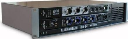
**iDR0 MiniRack** The MiniRack is similar to the iDR10 MixRack except it does not have any card slots for input or output modules. Instead it gets its audio via the EtherSound network. It can be used as the slave mix engine in an FOH/Monitor system with digital mic split, or as a compact mixer with an iLive modular Surface using the audio I/O in the back of the Surface.
