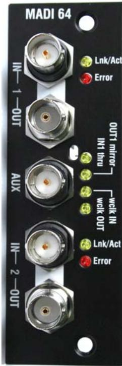
**MADI** (Multichannel Audio Digital Interface) is an industry standard multiple channel audio interface documented by the Audio Engineering Society as AES10. The **M-MADI** option supports 64 channels of **48kHz** serial digital audio transmission over 75 ohm coaxial cable to a maximum cable length of up to 150 meters (500 feet) depending on equipment connected and cable type used.
