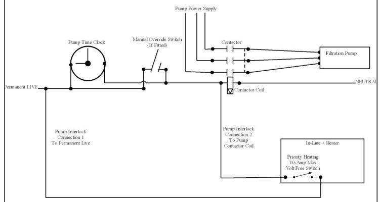
**NOTE** - Do <u>NOT</u> connect the pump interlock cable directly to the swimming pool pump as this will result in overloading the heaters digital controller.
