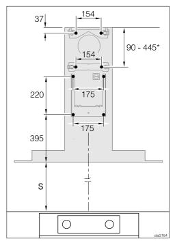
■ For pre-installation of a back wall where the holes have to be predrilled, please refer to the drilling distances in the drawing above (screws Ø 5 mm).
