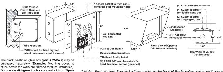
\* **Note:** Peel off paper liner and adhere gasket to the back of the faceplate, centering it over the four corner mounting holes.
