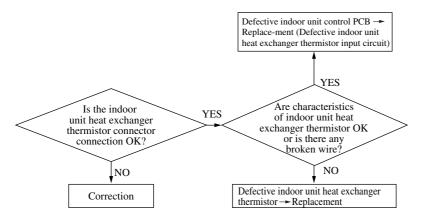
Return air thermistor (Th<sub>1</sub>A) Indoor unit heat exchanger thermistor (Th<sub>1</sub>R1, R2) Resistance temperature characteristics
