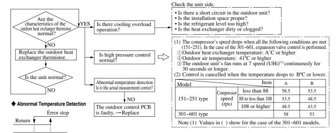
Note (1) In the case of the 151 ~ 251, the abnormal stop temperature differs depending on the compressor's speed.
