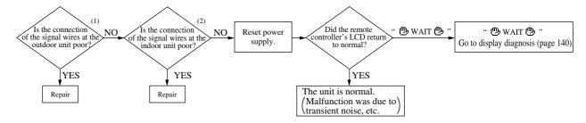
Notes (1) Check for poor connections (disconnection, looseness) on the outdoor unit's terminal block.
