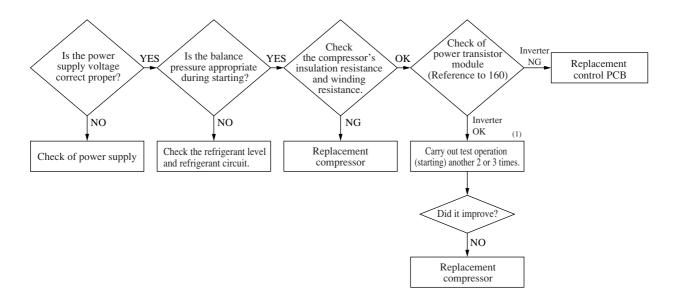
Note (1) If the test operation is repeated 2 or 3 times, the liquid refrigerant inside the compressor may be expelled from the compressor may recover from its starting abnormality.
