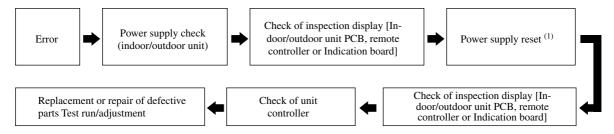
Note (1) It means the operation to turn off the power and back on again more than 1 min. later in order to reset the malfunction of microcomputer due to the effect of power supply conditions or accidental noise.
