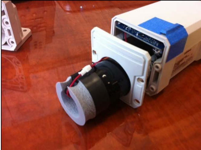
Figure 21: Reconnect Power Cables
