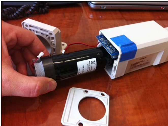
Figure 20: Proper Alignment to Slide Battery Out and In of Enclosure
