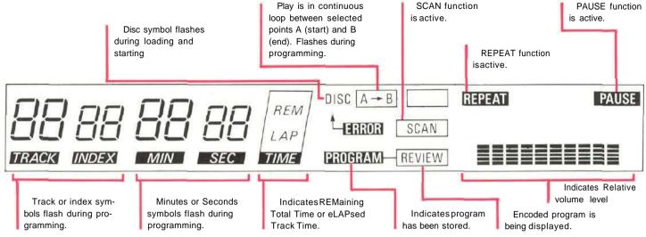
The display in the message center presents many different types of information. As soon as the POWER button is touched to turn the player on, the message center shows a series of zeros in TRACK, INDEX and TIME. The eLAPsed time indicator and the VOLUME bar are also lighted.
