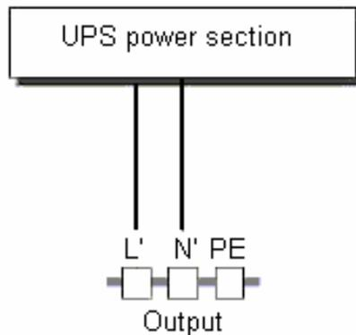
Figure 2: Connection diagram
