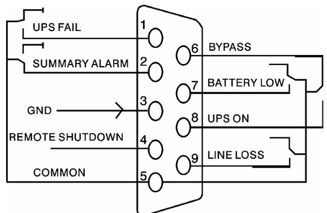
Figure 16.2: DB-9 Interface of AS400 communication protocol
