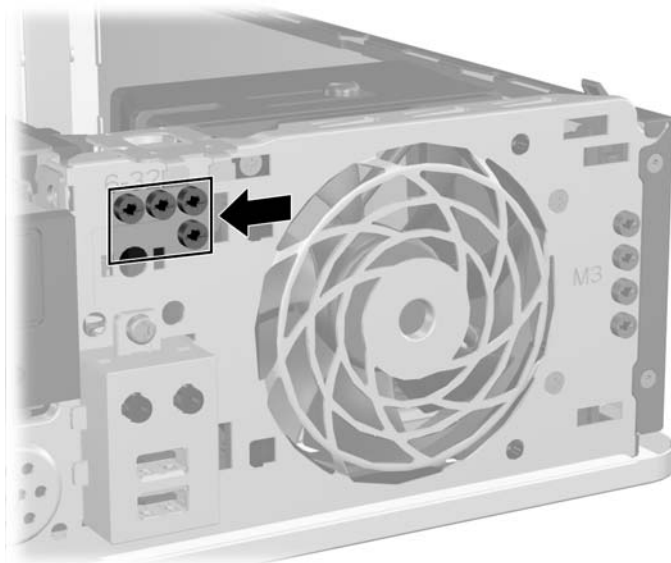
Figure 2-19 Secondary Hard Drive 6-32 Guide Screws Location
