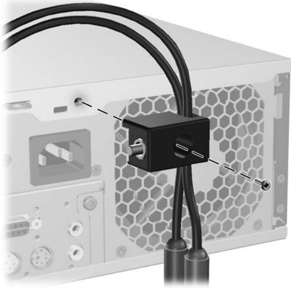
Figure C-5 Attaching the Lock to the Chassis
