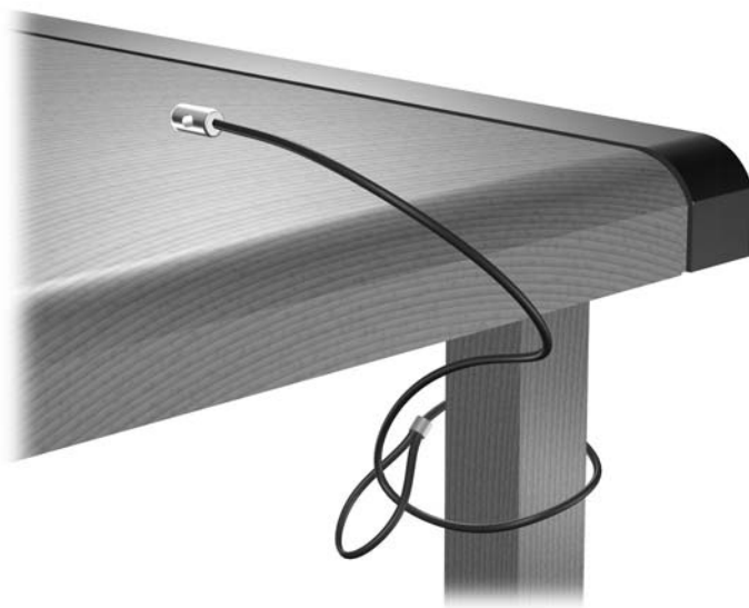
Figure C-3 Securing the Cable to a Fixed Object
