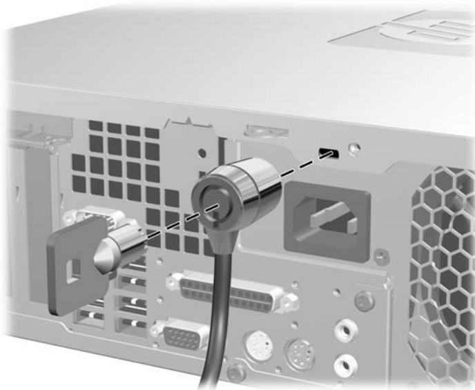
Figure C-1 Installing a Cable Lock
