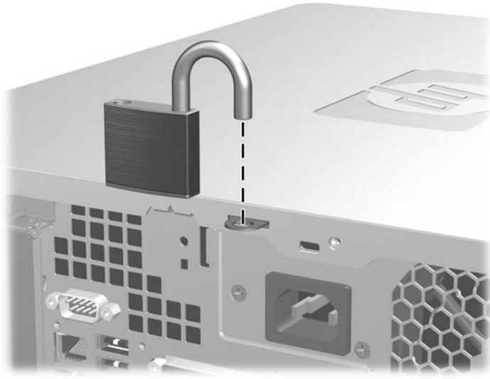
Figure C-2 Installing a Padlock
