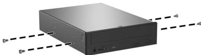
Figure 2-26 Installing Guide Screws in the Optical Drive
