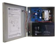
The AL125UL is a power limited power supply/charger that will convert a 115 V AC input into two individually PTC protected 12 V DC or 24 V DC outputs. They are
