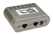
Microsemi's PowerDsine PD-AS-701 high-power active splitters enable data terminals that were not originally designed to accept Power over Ethernet, to be powered by HiPoE switches and midspans. The PD-AS-701 high-power series (12 V, 18 V and 24 V) can power devices such as WiMAX CPEs, small WiMAX base stations, 802.11n access points, thin clients, PTZ IP cameras, video phones and more.
