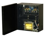
These remote accessory modules link to HubWay passive and active UTP transceiver hubs and transmit video from up to four cameras over a single Cat 5 structured cable. They provide local power to cameras which eliminates voltage drop due to long cable runs. Unit can be utilized as a stand-alone passive UTP transceiver hub with integral camera power.
