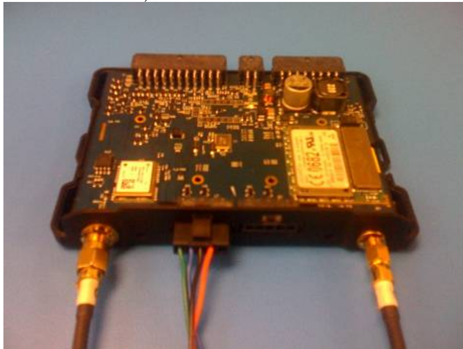
Figure 5 - LMU-4200™ Serial Cable Plugged into Aux 1
