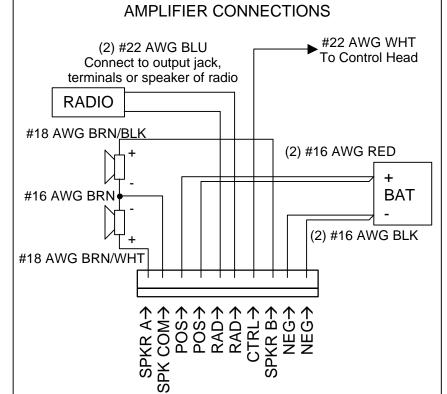
Attach leads by stripping 3/8", inserting into connector and clamp by tightening screw. Make sure the screw is tight and the wire can't be pulled out. Failure to adequately tighten the screw can result in improper operation or burning the connector and wire.
