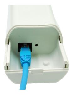
**Figure 4 Cable Connection**
