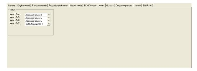
Here you can assign functions to the switching-inputs.
