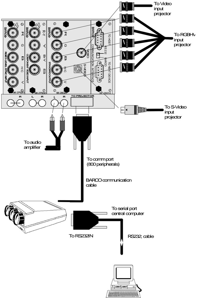
Plug the female D9 connector of a serial cable into the male connector of the serial port of your computer.
