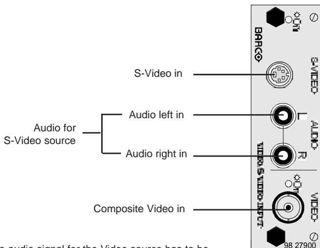
The audio signal for the Video source has to be connected to the audio input just below the Video input slot.
