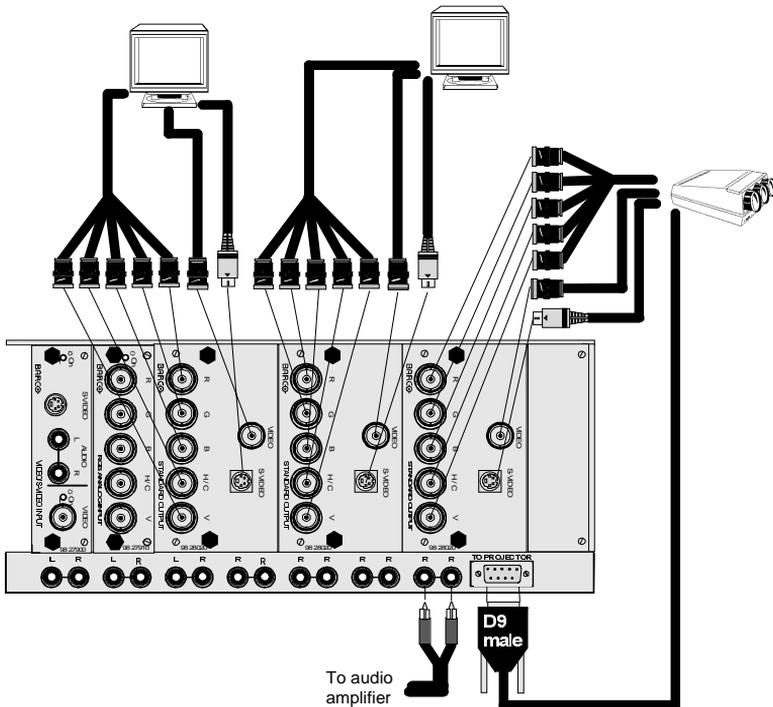
RCVDS05 to the Red, Green, Blue, H/S sync and V sync inputs of the display 1 using coaxial cable with BNC connectors.
