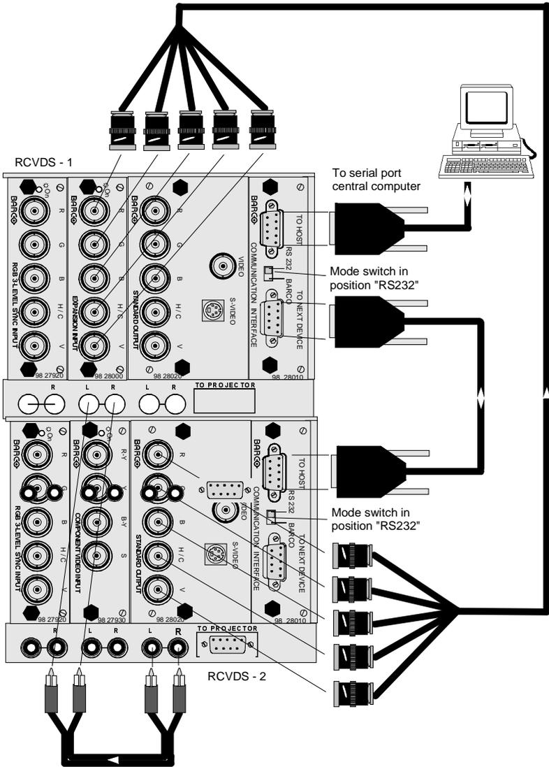
the second RCVDS05 and the audio connectors below the expansion module of the first RCVDS05.
