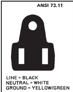
The wires of the power cord are colored in accordance with the following code.
