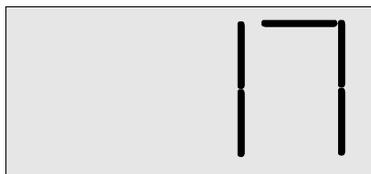
Only the first RCVDS will indicate the source number on its display. All others RCVDS's will display a double point. The optional IR receiver, if connect, will always display the source number.
