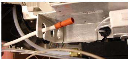
Figure 8 Connecting the APCI HV to the chassis.
