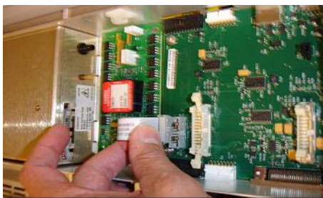
Figure 4 Connecting the valve PCA to the multimode HV power supply.
