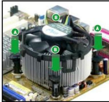
3. Connect the CPU fan cable to the connector on the motherboard labelled **CPU\_FAN1**.
