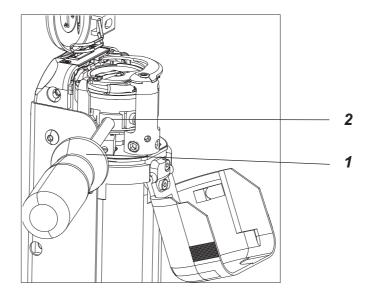
When the thread gets jammed in the hook track, the safety clutch disengages.
