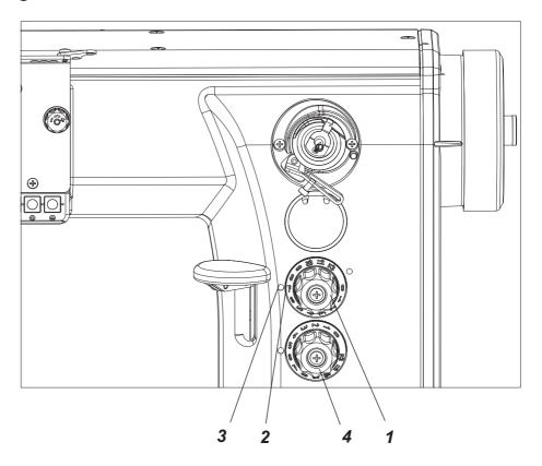
The special sewing machine 838 is equipped with two setting wheels. This allows you to sew with two different stitch lengths which can be activated during the sewing process by pressing a button.
