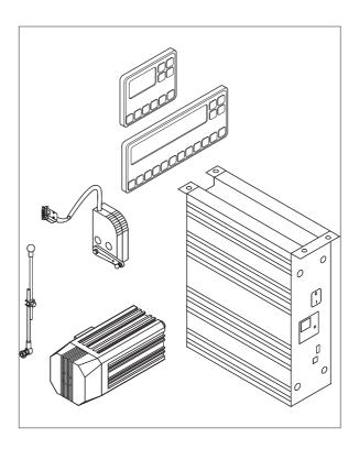
The DA321G control unit contains all required operational interfaces for switching functions and setting parameters. It is possible to operate without an operating panel, but the seam programming can no longer be carried out.
