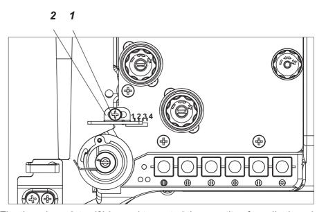
The thread regulator (2) is used to control the quantity of needle thread required by the stitch formation.
