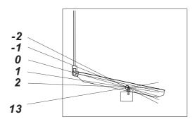
The pedal position is detected by a button with 16 different levels. Their meanings are listed in the table below:
