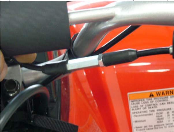
Step15-Fig1-Throttle cable free play adjustment
