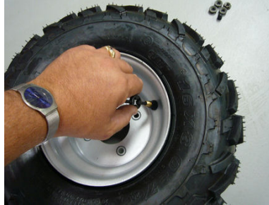
Step4-fig2 Tightening valve core with core tool
