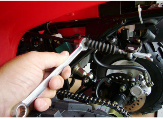
Step15-Fig2-Rear brake cable adjustment
