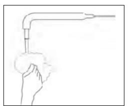
ATTENTION: The probe must NOT be washed with boiling water.
