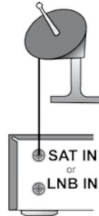
Connect the Receiver to the LNB on the dish.
