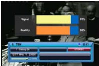
This screen shot indicates that the receiver is connected to a LNBF. The meters show that there is good Signal Level and good Signal Quality readings.
