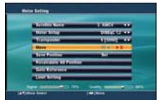
All DiSEqC 1.2 saved satellite motor positions can be globally shifted or offset with RECALCULATE ALL POSITION command.
