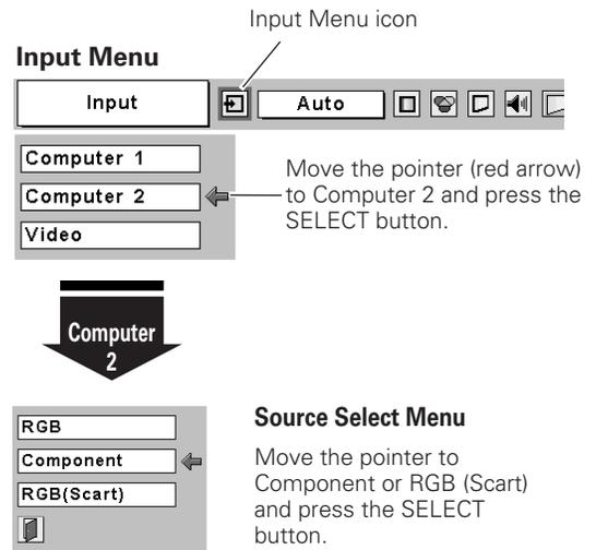
**Component** When the input source is coming from video equipment connected to the COMPUTER IN 2/ COMPONENT IN/ MONITOR OUT terminal with a Component-VGA Cable, select Component.
