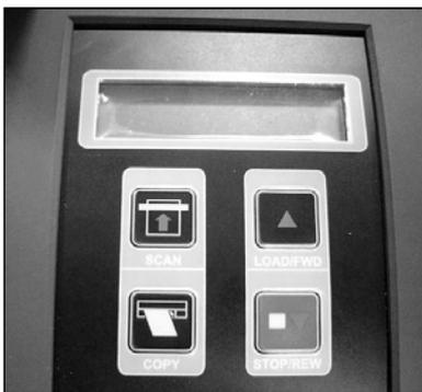
SmartLF Cx can now be switched on. The liquid crystal text display (LCD) will light up and after a few seconds will display the word 'Initialising'. After about 35 seconds or so the model number and firmware level of the scanner will be displayed.
