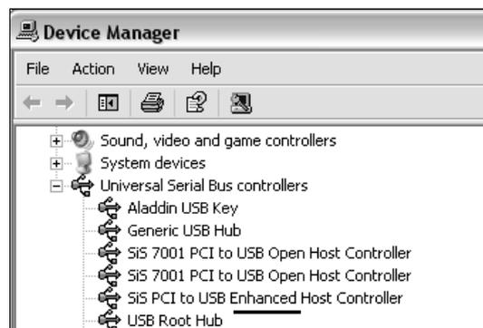
NOTE: Every port can potentially have a different version of the SmartLF Cx driver loaded for it so if you have recently upgraded the driver for SmartLF Cx and changed the USB port you regularly connect through you should check the driver level using the Properties tab. Always reboot after updating a USB driver.
