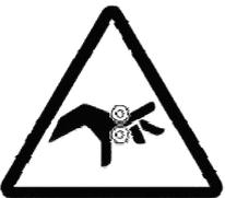
This symbol is intended to alert the user to the presence of important operating and maintenance instructions. The equipment being used constitutes a potential finger trap and could cause personal injury.
