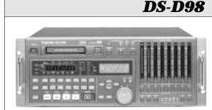
The DS-D98 is the only tape-based recorder that supports Sony's Direct Stream Digital (DSD) for Super Audio CD (SACD) creation. DSD recording uses a 2.8224 MHz sampling frequency for the original 1-bit data to allow
