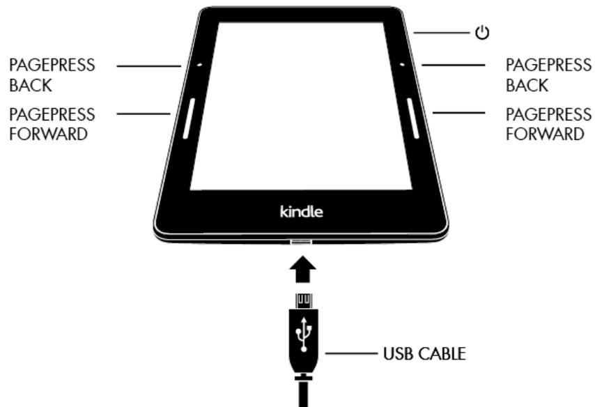
**PagePress:** To page forward or back in a book, squeeze either side of the screen. Use the line to page forward and the dot to page back. You can keep your right or left thumb resting on the pressure-sensitive controls. To adjust the pressure required to turn a page or the feedback you receive when a page turns, go to Settings, Reading Options, then PagePress.
