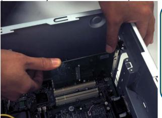
To avoid damage caused by static electricity, make sure to properly ground yourself by first touching a metal part of your computer to discharge any static electricity before working with the DWL-520+ Wireless PCI Adapter.
