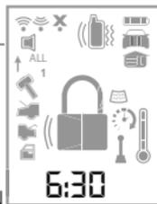
If the door was open when locking, you are notified of an active zone immediately after locking the system. The horn in the vehicle “honks” again. The 2-way remote control sounds a short “error” tone, and the LCD displays the door icon.
