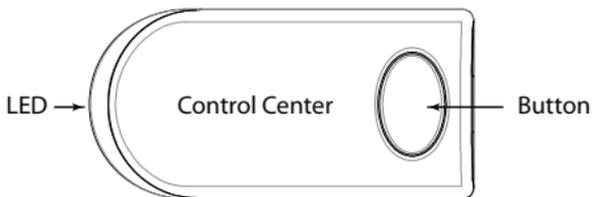
The Control Center, typically located on the upper part of the front windshield sends and receives commands or messages to and from your system. It consists of:
