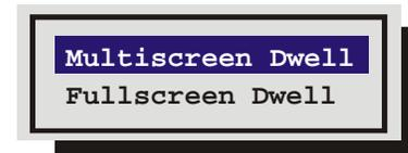
The dwell time is the amount of time each camera is displayed on-screen (while sequencing) before advancing to the next camera.
