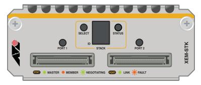
The following LEDs report operations and faults on the XEM-STK.
