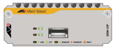
The following LEDs report operations and faults on the XEM-1XP.
