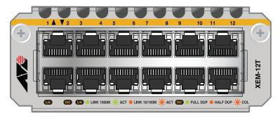
The following LEDs report operations and faults on the XEM-12T.
