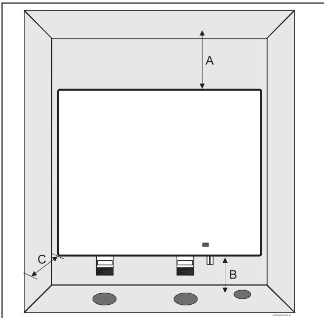
Fig. 5 Recommended minimum clearances
